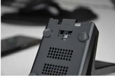
The first thing to do if you want to make recordings, you insert the micro SD card into this slot in DVR. To access the SD card compartment is necessary to open the cover into the base by sliding it sideways.
